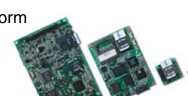
T-Engine Platforms (Standard T-Engine, micro T-Engine, nano T-Engine, pico T-Engine)
